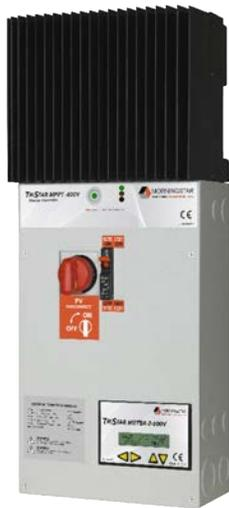
Morningstar's TriStar MPPT 600V charge controller is available with and without a DC Disconnect Box. Model TS-MPPT-60-600V-48-DB includes a compact on-board DC Disconnect Box, which helps to save on installation time and cost. The DC Disconnect Box enables the TriStar MPPT 600V charge controller to be used in either positively-grounded or negatively-grounded PV systems. The DC Disconnect Box includes the following features:
