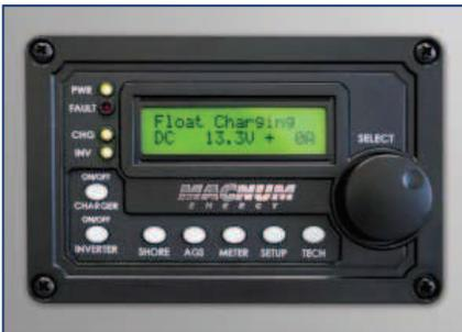
The ME-RC is designed to be simple to use while offering multiple functions in one place. It includes an easy-to-read LCD screen, at-a-glance LEDs, non-volatile memory, and works with all Magnum inverters.
